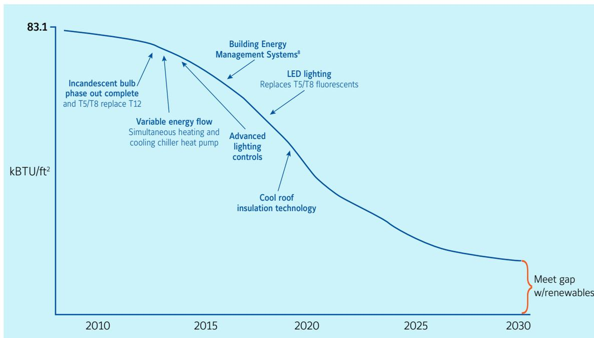
\* System comprised of demand response capability, energy performance monitoring/ analytics, and integration of component-level controls and sensors.
