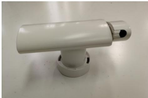
The Comfort Eye is an innovative comfort sensor equipped with a low-cost IR sensor, installed on the ceiling or wall and capable of motorized pan and tilt to measure the indoor surfaces temperature. A central unit manages the IR scanning process, calculates the mean radiant temperature and finally the PMV comfort index (according to ISO 7730) using on board sensors.
